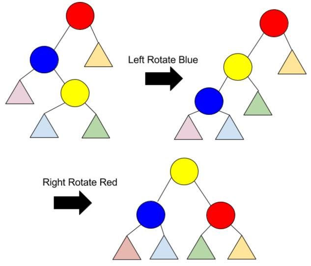
insertion: insert as normal then rebalance deletion: delete as normal then rebalance search, min, max, successor, predecessor - same as BST Time to rebalance after insert or delete is O(log(n)) => insert, delete O(log(n))
